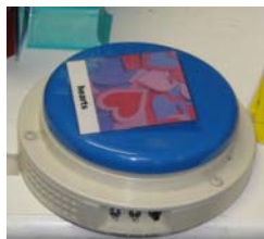
figure 6. An oversized button providing mediated speech functionality
