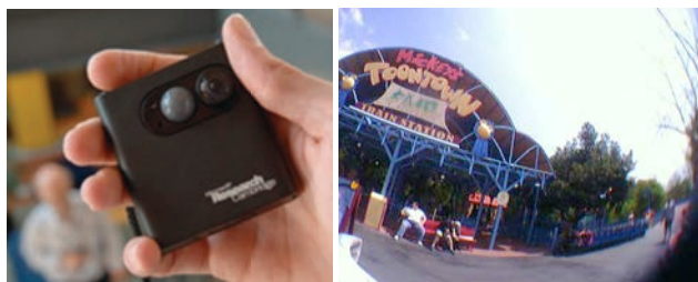
Figure 1. (left) The SenseCam form factor used in this study; (right) Sample SenseCam image.
